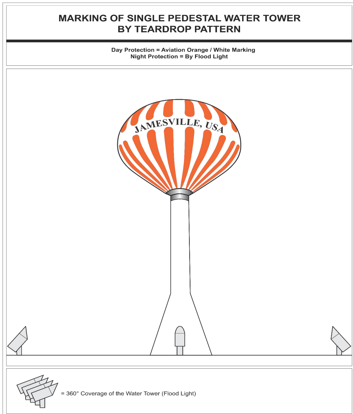
Figure A-5. Marking a Single Pedestal Water Tower Using the Teardrop Pattern
